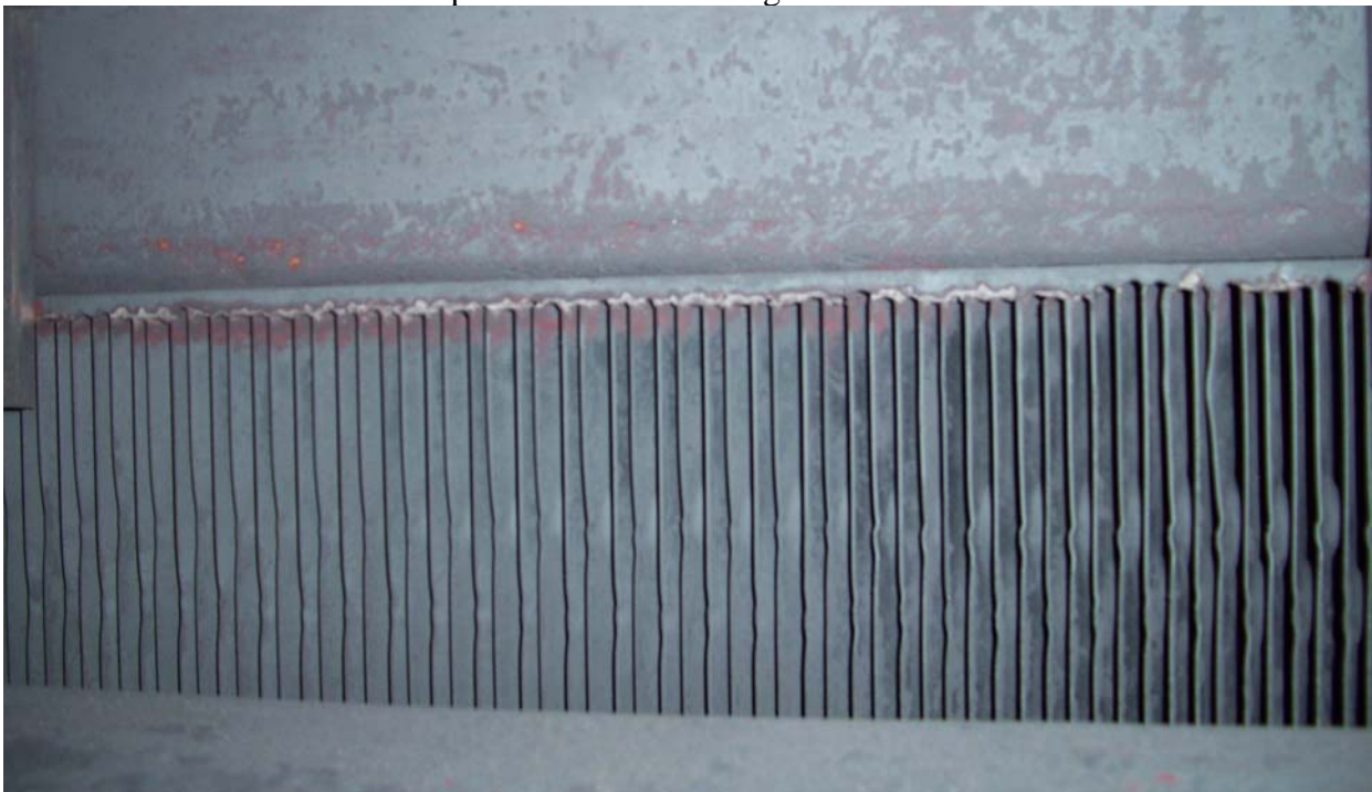
Photo 4: The presence of whitish marks along the edge of the primary drier in the steam space.
